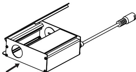
4. Insert the electrical supply cable through the knockout and secure with a cable connector. Wire driver box (Fig.3), white - white, black - black, green - green/ground.
