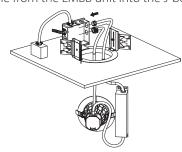
c. In the J-box, use wire nuts to do the wire connections as illustrated in the diagram below. If the purple (DIM+) and grey (DIM-) wires from the downlight are not in use, cap these with wire nuts. If the test switch is not in use, cap the purple (Test +) and brown (Test -) wire from the EMBB with wire nuts. Make sure EMBB is grounded. (Fig.24)
