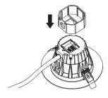
4. Adjust dial settings on the Emergency Battery Backup System (EMBB) for desired output current. Reference EMBB List table.
