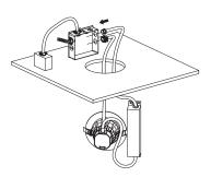
c. In the J-box, use wire nuts to do the wire connections as illustrated in the diagram below. If the purple (DIM+) and grey (DIM-) wires from the downlight are not in use, cap these with wire nuts. If the test switch is not in use, cap the purple (Test +) and brown (Test -) wire from the EMBB with wire nuts. Make sure EMBB is grounded. (Fig.29)
