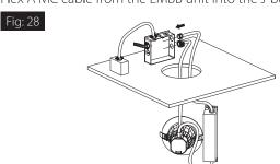
c. In the J-box, use wire nuts to do the wire connections as illustrated in the diagram below. If the purple (DIM+) and grey (DIM-) wires from the downlight are not in use, cap these with wire nuts. If the test switch is not in use, cap the purple (Test +) and brown (Test -) wire from the EMBB with wire nuts. Make sure EMBB is grounded. (Fig.29)
