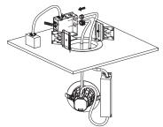
c. In the J-box, use wire nuts to do the wire connections as illustrated in the diagram below. If the purple (DIM+) and grey (DIM-) wires from the downlight are not in use, cap these with wire nuts. If the test switch is not in use, cap the purple (Test +) and brown (Test -) wire from the EMBB with wire nuts. Make sure EMBB is grounded. (Fig.24)
