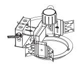
6. Remove the existing lamp metal conduit (MC) cable from the J-Box. (Fig.5)
