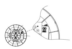
4. Insert screws into J-Box holes, leaving about 15mm of space between the screw heads and J-Box. (Fig.3)
