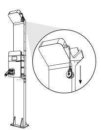
a. Refer to cable outer diameter to select appropriate inner ring (D18 or D22) for cable clip.
