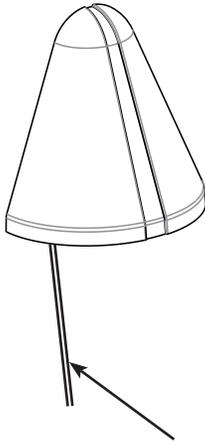
Use UL approved wiring connectors for SPT-1 cord
