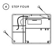
Mount the Gateway to the installation surface using size 10 screws appropriate for the surface material. For direct installation onto an external junction box, use the junction box's included screws.
