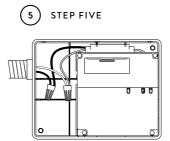
Install included battery with negative (-) end facing towards junction box area. Call RAB to request replacement rechargeable batteries.
