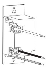
Use the two 6-32 1/2" Phillips round head screws to secure the Dimmer to the junction box.
