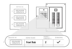
For setup and maintenance, we provide two Lightcloud Device Tables with the Gateway: one that you can attach to your panel and one to hand off to a building manager. Attach the Device Identification stickers included with each device to a row, then write in additional information, such as Zone name, Panel/Circuit Number, and whether or not a zone uses dimming.
