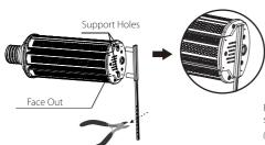
For face-out installation use the one-legged support and cut to desired length (Fig.5)
