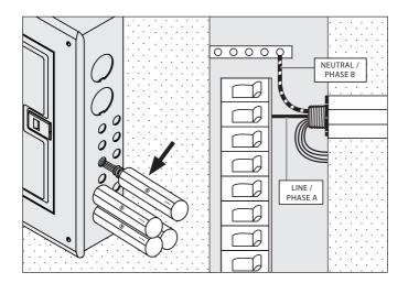
Space and code allowing, you may install Lightcloud devices directly in your breaker box or lighting panel. Alternatively, break out lighting circuits and install Lightcloud devices in a separate trough.
