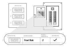
For setup and maintenance, we provide two Lightcloud Device Tables with the Gateway: one that you can attach to your panel and one to hand off to a building manager. Attach the Device Identification stickers included with each device to a row, then write in additional information, such as Zone name, Panel/Circuit Number, and whether or not a zone uses dimming.
