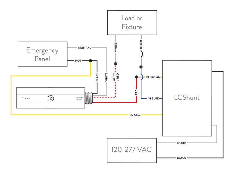
**Note:** The LCSHUNT includes a 20A rated high voltage Form C (N/O+N/C) relay and is UL924 Listed for emergency lighting control applications. The LCSHUNT can bypass a line voltage switch or dimmer, ensuring that an emergency fixture illuminates at full brightness during a utility power interruption.
