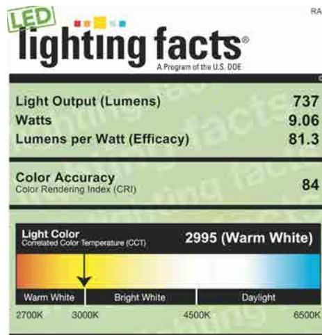
All results are according to IESNA LM-79-2008: Approved Method for the Electrical and Photometric Testing of Solid-State Lighting. The U.S. Department of Energy (DOE) verifies product test data and results.
