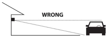
**Solution:** A 20ft safety zone and lower sensitivity are recommended to avoid activation from passing cars.
