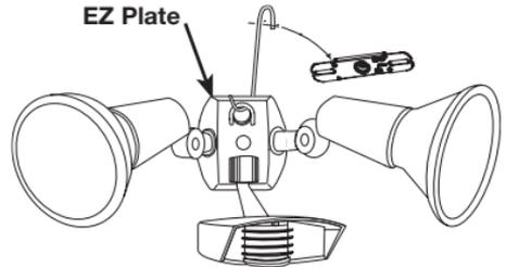
1. Attach the Universal Mounting bar with the bar screws (provided) to the junction box. If you are attaching your STL110 kit to a surface mount weatherproof box, you must use both gaskets, with the metal mounting plate
