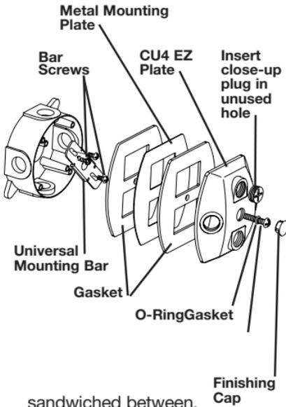
3. Bring power leads and sensor kit leads through holes in all gaskets into junction box.
