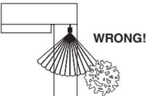
**Solution:** (1) Aim sensor away from movement or (2) mask lens as in the direction of the source and/or (3) lower sensitivity control setting.
