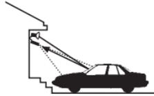
Solution: Aim sensor away from reflective objects, or move the objects and lower sensitivity.
