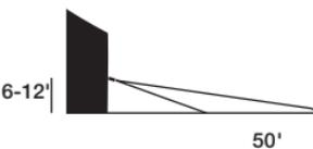
3. Check that movement is not directly towards sensor. Sensor will see movement across its pattern more quickly. To fix, move the sensor.
