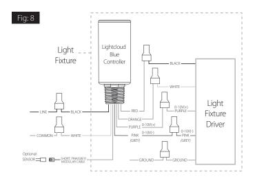
**NOTE:** Do not connect DIM V+ (purple)/ DIM V- (pink(grey)) to line voltage or supply ground.
