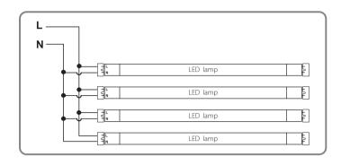
The below ballast wiring represents typical configuration. The actual ballast wiring varies according to ballast model. It is not needed to change socket (if in good condition) to operate double ended lamps, regardless the type of sockets. Please make sure one side of fixture is connected to Live (L) and the other side to Neutral (N).
