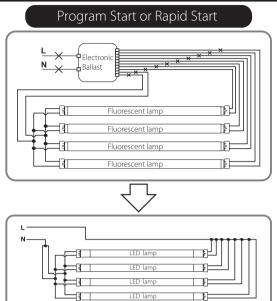
The units covered by this report were intended to retrofit surface mount, Type IC or non-IC recessed mount Listed fluorescent luminaires that use maximum four or six tubular lamps. The minimum lamp compartment dimensions are tabulated below:
