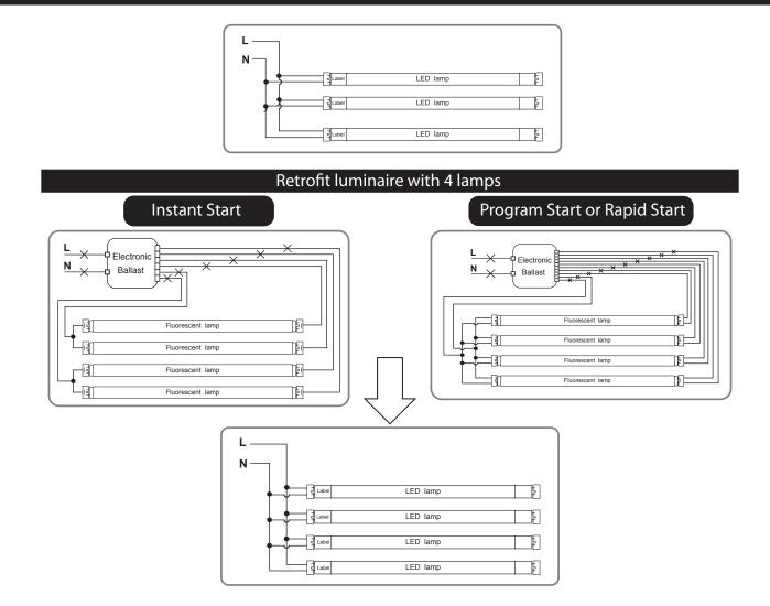
The below ballast wiring represents typical configuration. The actual ballast wiring varies according to ballast model. It is not needed to change socket (if in good condition) to operate double ended lamps, regardless the type of sockets. Please make sure one side of fixture is connected to Live (L) and the other side to Neutral (N).
