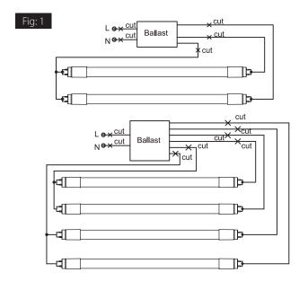
3. Wiring the driver as following figures, (Fig. 2) the LED tube designed can be both single end input or double ends input.
