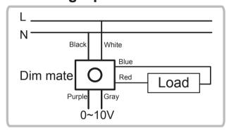
0-10V Continuous dimming by selected Dim-mate&Dimmer Kit in the package,Operation refer to the wiring diagram "Dimmable via an external accessory" in definition of DLC V5.1.
