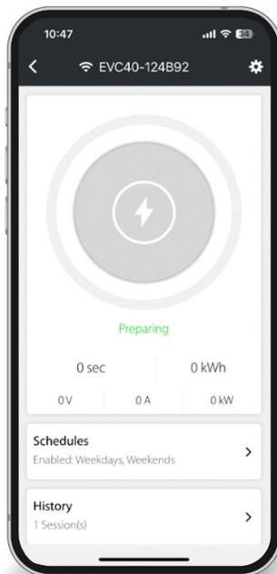
On the charger app screen, you'll notice the circular Start/Stop button. If the charger is not charging, the circular Start/Stop button will be grayed out.
