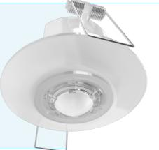
This passive infrared motion detector can be installed into a drop ceiling to control individual or grouped fixtures. Simply connect the sensor to a compatible Lightcloud Blue Controller using the RJ09 connector. Once paired, the sensor can be programmed for Occupancy or Vacancy, set timeouts, sensitivity levels, and specify actions.
