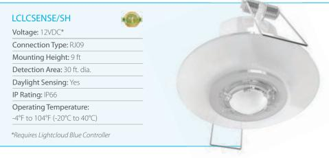
This passive infrared motion detector can be installed into any ceiling to control individual or groups of fixtures. It functions as both an occupancy and vacancy sensor and also acts as a daylight harvester.
