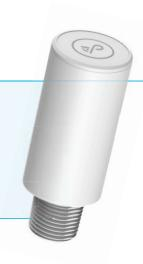
Turn any 0-10V LED fixture into a Lightcloud Blue-enabled luminaire with a Lightcloud Blue Controller. It's easily attached to a 1/2" knockout on the fixture or a j-box, or can simply be factory-installed onto your favorite compatible RAB fixture. The Controller's button can also be used to identify the device within the app, to turn the fixture on/off, and to set dimming level.
