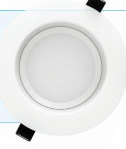
This high-performance, 18W downlight is optimized for both new construction and retrofit applications, with a universal, 120-277V onboard driver and 0-10V dimming. Adjustable, springloaded retention tabs keep the fixture secure after installation, and extension ring accessories make it easy to use the 6" downlight in 8" housings.
