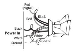
Red pigtail is only used to switch remote or additional fixtures.
