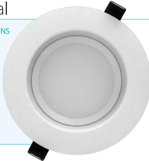
This high-performance, 18W downlight is optimized for both new construction and retrofit applications, with a universal, 120-277V onboard driver and 0-10V dimming. Adjustable, spring-loaded retention tabs keep the fixture secure after installation, and extension ring accessories make it easy to use the 6" downlight in 8" housings.
