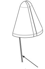
Use UL approved wiring connectors for SPT-1 cord
