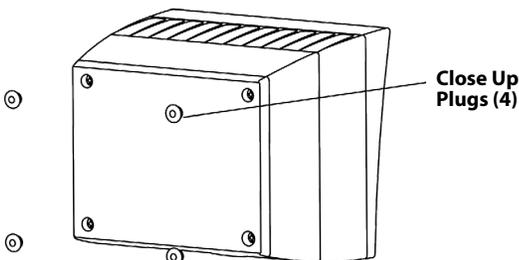
If desired, cover the screw holes with the provided **Close Up Plugs** (4) on the back cover as shown above. Tap lightly into place.
